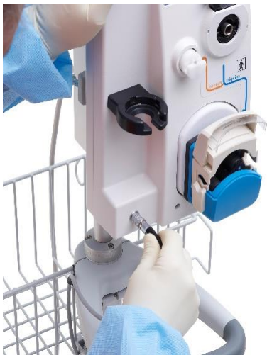
Figure 12 Foot Control Connection
