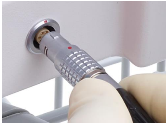
Figure 13 Alignment of Red Dots
