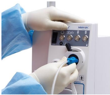
Figure 15 Inserting Catheter proximal housing
