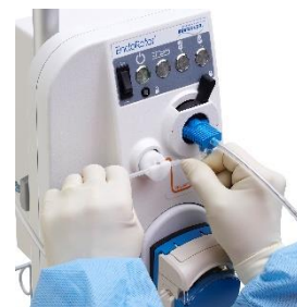
Figure 20 Tubing insertion
