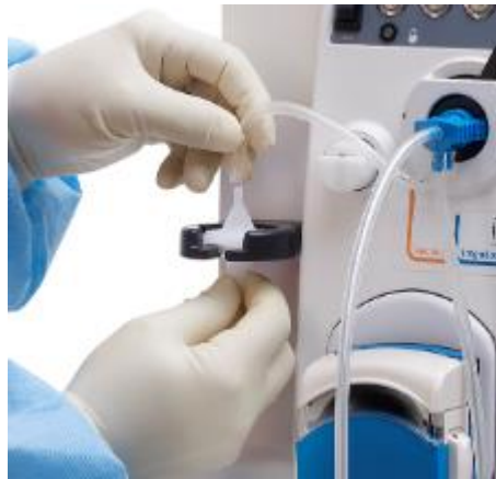
Figure 22 Raccordement du tube d'aspiration
