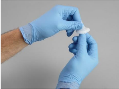
Figure 8 Counter rotate trap halves
