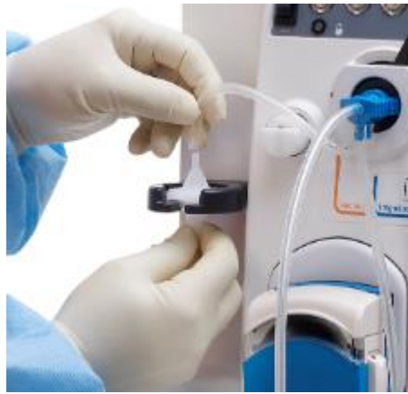
Figure 22 Connecting Vacuum Tube
