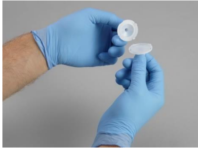
Figure 9 Separate Trap halves
