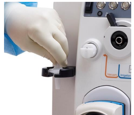
Figure 14 Placement of Specimen Trap
