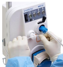
Figur 20 Slange settes inn
